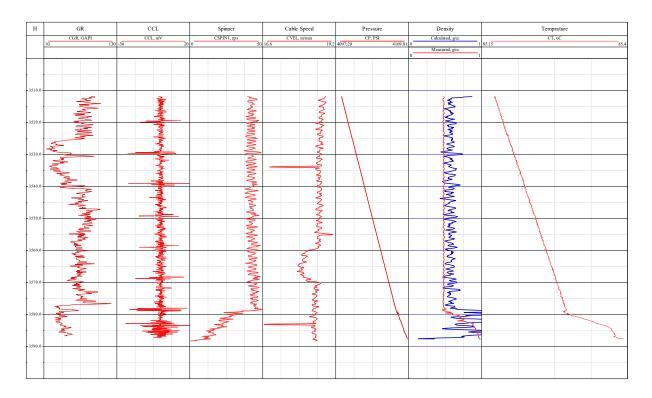
The TFD data interpretation is more accurate and less noisy compared to the calculated density from the pressure gradient (same as column 6 on the chart above), allowing better distinction of fluid phases and constructing an accurate production profile.
