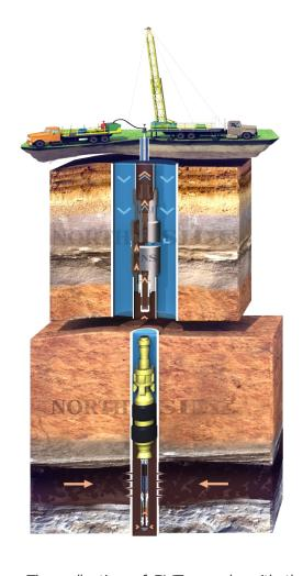
Drill stem test with a jet pump is the best way to test multilayer formation zone by zone creating variable drawdown to the reservoir to evaluate its performance at different flow regimes.
