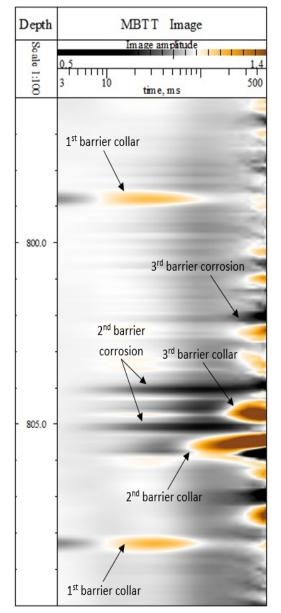
The calculation of the metal loss percentage each particular pipe is based on the behavior of the most relevant **EMF** decay curves comparison with baseline corresponding to a nominal pipe thickness. The North Side inhouse software allows for determining the best match between the recorded data and the calibration database coming from the real field tests.
