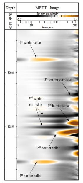
The calculation of the metal loss percentage of each particular pipe is based on the behavior of the most relevant **EMF** decay curves comparison with baseline corresponding to a nominal pipe thickness. The North Side inhouse software allows for determining the best match between the recorded data and the calibration database coming from the real field tests.
