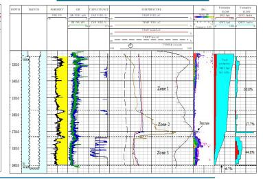
HPT. Spinnerless Production Profiling
